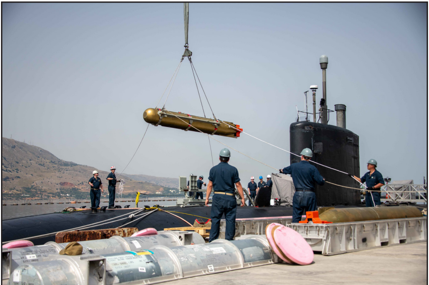
Sailors aboard the Los Angeles-class submarine USS Montpelier (SSN 765) conduct an expeditionary ordnance on-load in Souda Bay, Greece, exercising the capability to load the MK 67 submarine launched mobile mine.
