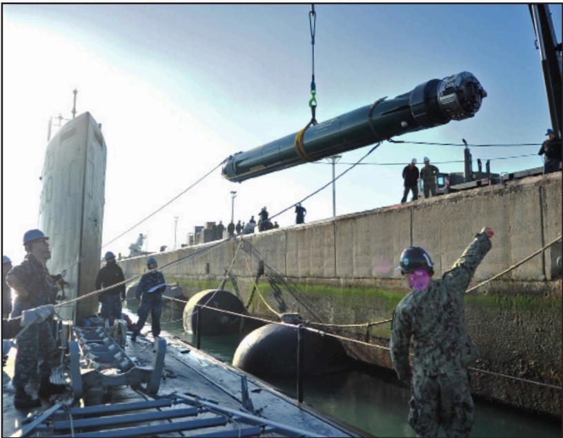
An MK 48 inert training torpedo is loaded aboard the Virginia-class submarine USS California (SSN 781).
