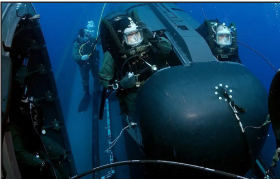
The SEAL Delivery Vehicle (SDV) Mk 8 seen above is a "wet" swimmer delivery vehicle.
